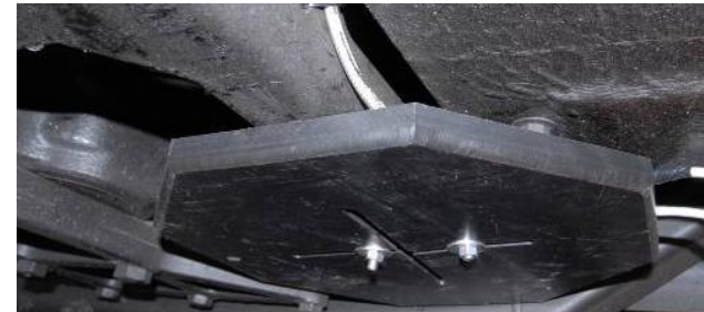
Aerial mounted on tram underside
